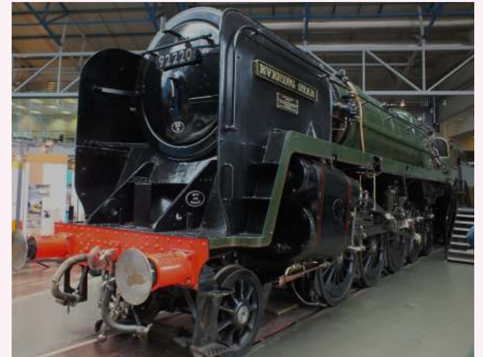
Last steam loco built by British Railways. 9F Class 2-10-0 No 92220 Evening Star at the National Railway Museum, York. (Photo credit Paul Whittle)
