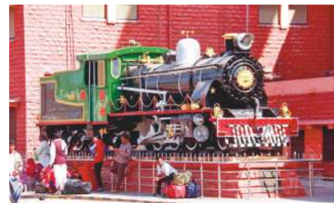
► 1959 built ZB class NG loco, Duro Dakovic, Slavonski Brod, Yugoslavia. No 120. Now at Jodhpur Railway Station
