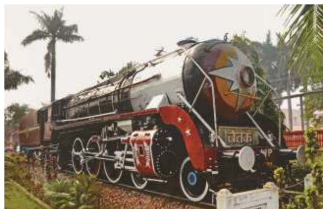
1955 built WP class BG loco, Canadian Locomotive Company, Ontario. No 7581. Now at DRM office Sonapur
