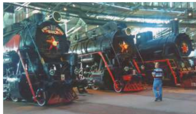
On the left L 2298-4199 built between 1945-55. This locomotive was built in honour of the 12th Congress of Komosol (Youth Congress). In the center is LV - 18-002 Main freight locomotive successfully developed during World War II. It had a thermal efficiency of 9.27%
